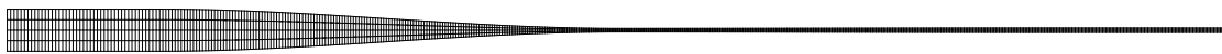
Figure 6. Mesh of the nozzle corresponding to the case with \mathcal{M}_1 = 0.050 and \mathcal{M}_2 = 1.600 .
